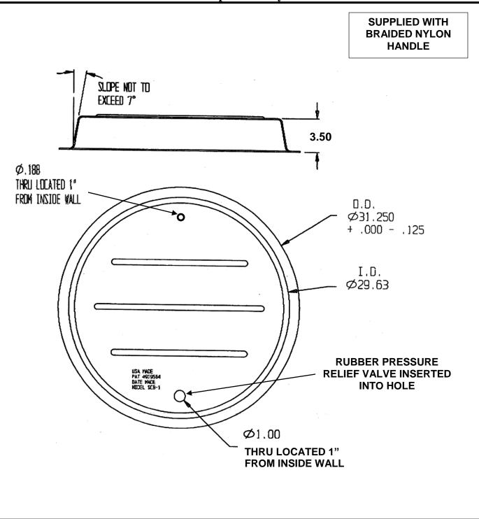
STAINLESS STEEL 'RAINSTOPPER' MANHOLE INSERT (SIZE 'SCB-1')
